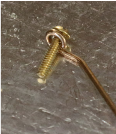
Figure 2: Loop and bend
