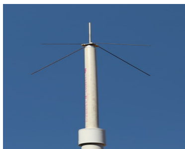
Figure 1: 442 MHz Ground Plane Antenna Here is a list of materials:
